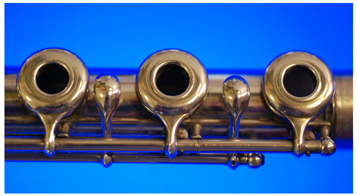
Louis Lot #136, with body numbered 186. Lot had to completely redesign the keywork when he left Godfroy's, yet he retained the original mechanics, including the shoulder clutches seen here.
