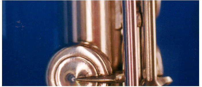
The thumb key, with original kickers showing the flute was made with a Bb trill, and has not been altered.
